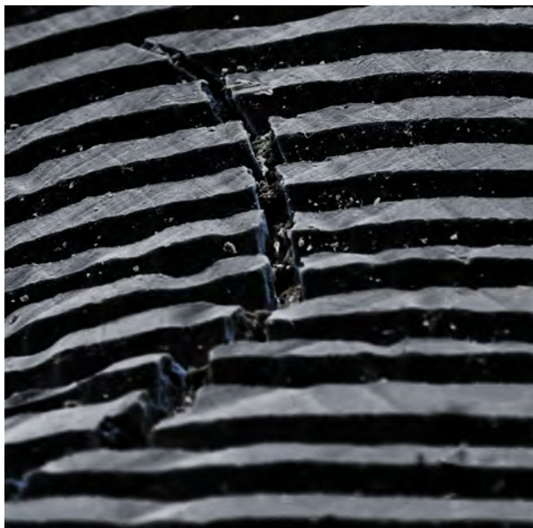
From the series From the Pit of Et Cetera, Montserrat (a phono-archaeology), Fieldnote 22-03-21 — WD 14.6mm (x300 view of recovered vinyl via Electron Microscope).
